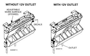
**NOTE:** The WorkStation can be attached anywhere in the platform unless the machine is equipped with another accessory, at which point the WorkStation must be attached on the opposite side.
