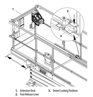
Figure 3-6. Platform Deck Extension (All Models)
