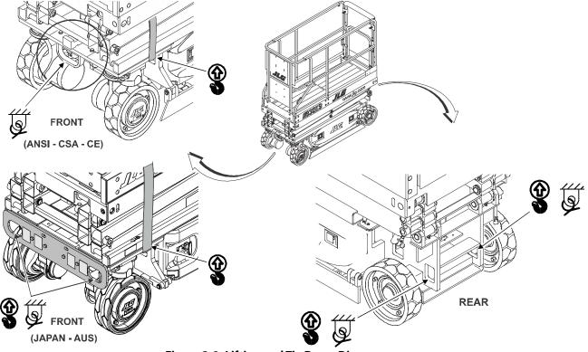
Figure 3-9. Lifting and Tie Down Diagram
