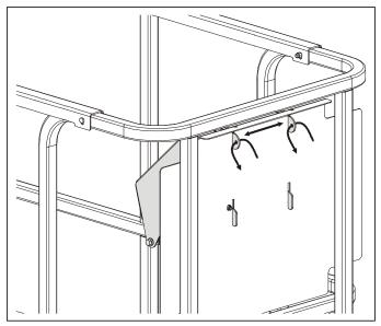
Figure 3-8. Securing Control Station to Platform
