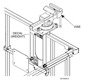
**NOTE:** If the WorkStation is installed, it must be mounted to the opposite side of the platform from the Vise.
