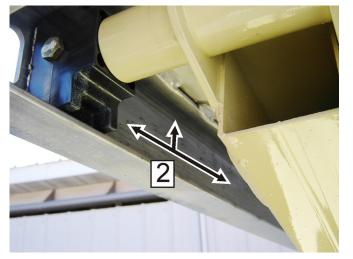
Figure 6-3. Upper Slide Pad Channel
