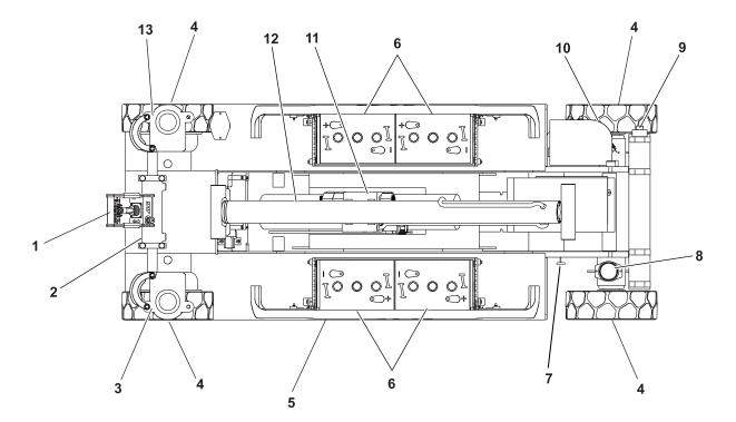
Begin the Walk-Around Inspection at Item 1, as noted on the diagram. Continue left (counterclockwise viewed from top) checking each item in sequence for the conditions listed in the following checklist.
