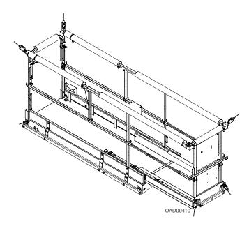
**NOTE:** Option with limit switches is shown.
